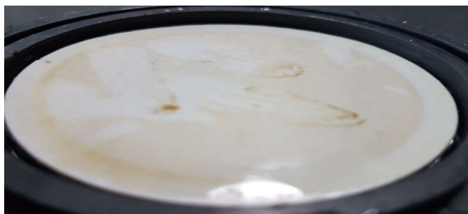
Fig.5. Clogging on the surface
