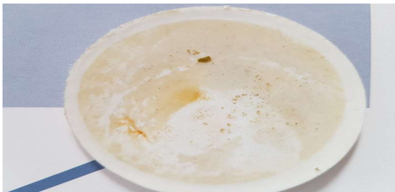
Fig. 8. Deposits on the membrane surface after filtration
